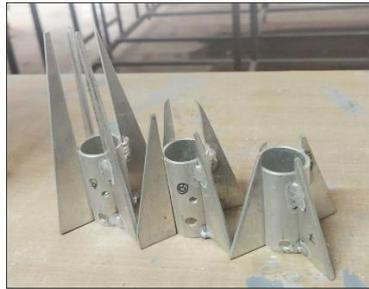
**Fig 7 : Attachable triangular 4 fins**
