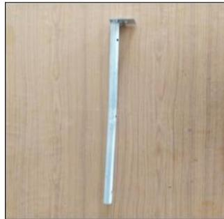
**Fig 5 : A Smooth Aluminum Pile****Table 2 : Dimensions of Pile**
