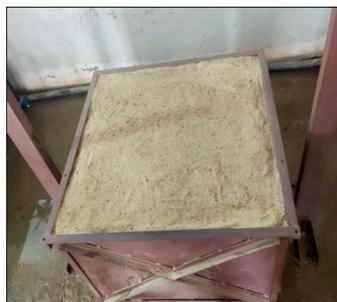
**Fig 9 : Sand Bed Prepared and Levelled**
