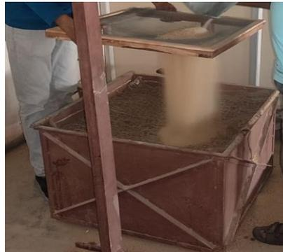
**Fig 11 : Sand Poured to the tank by Rainfall Technique**
