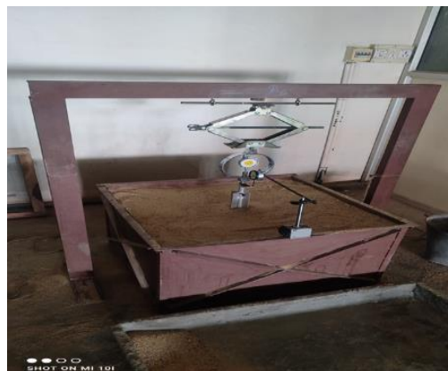
Fig. 9 : Sand bed prepared and leveled
