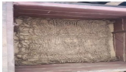
Fig 8 : Geojute in model tank
