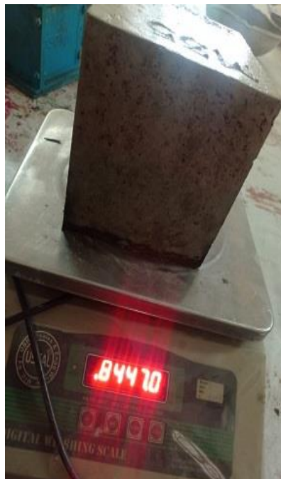
Fig. - 3 Water Absorption Test
