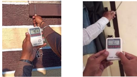
Fig 5: The temperature outside is 45.1 degree Celsius and the room temperature is 30.2 degree Celsius
