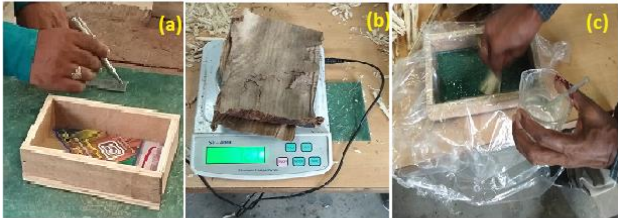
Fig. 1.2 (a) Preparation of wooden mould (b) weighing machine for measuring different raw materials used in composites and in (c) initial setup for composites is shown.
