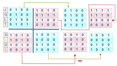
Here the diagonal and the anti-diagonal bit rotations are taking place as per the key mechanism. Now, after rotating the blocks we will concatenate the blocks and as well as the matrices to get the decrypted text.
