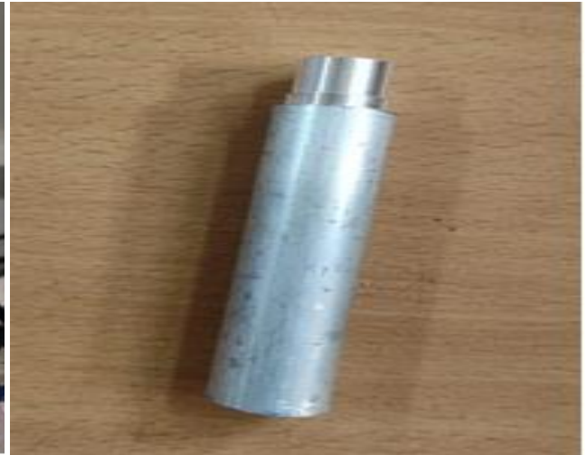
Fig.2: Aluminium workpiece after turning operation
