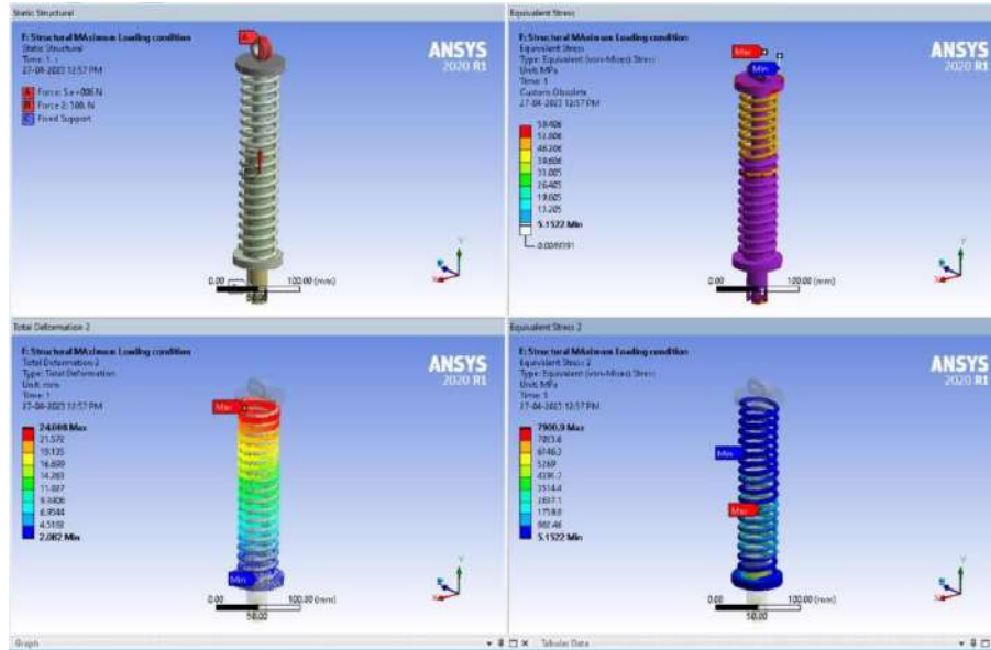
Figure No 21: Total deformation and Stress Factors of the spring part for Aluminum 700
