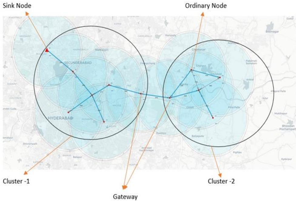
Figure: 4.1 MANET's capabilities in the Internet of Things to route packets from the source IoT end-device to the target via multiple cluster heads
