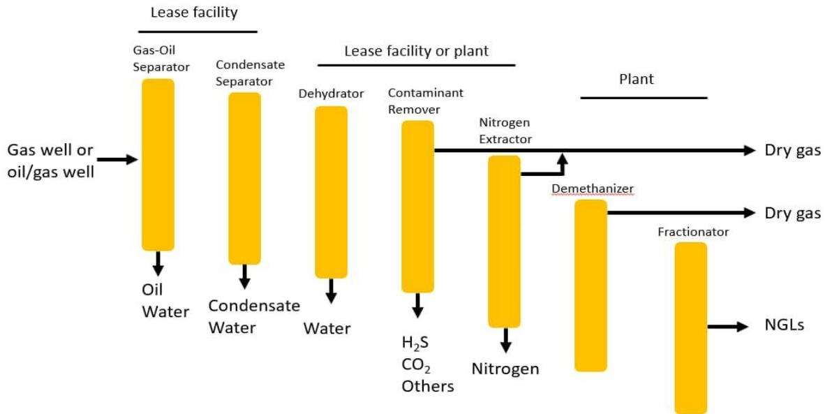
Fig 1. Illustrates the Gas Processing Flow
