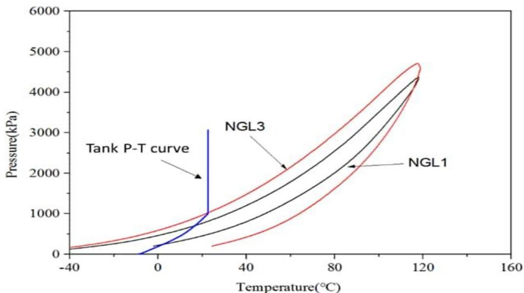
Fig 8: PVT (Pressure-Volume-Temperature) diagram specifically dedicated to the sub-cooling cycle.
