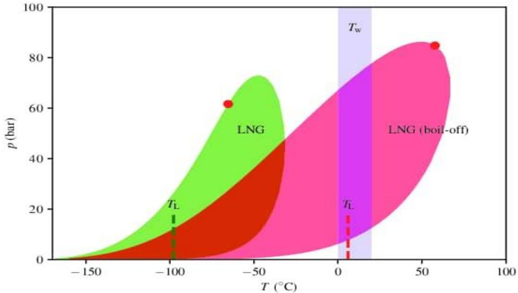
Fig 7: PVT (Pressure-Volume-Temperature) Diagram Specifically Designed for the Liquefaction Cycle.
