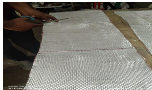
Fig (5.14) Cutting as per Marking
