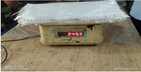
Fig (5.15) Measurement of GFRP Matt with 345.5 g
