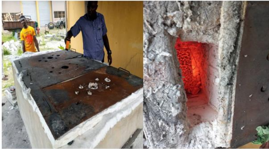
Plate 2. Calcination of Chikoko in Niger Delta University, Civil Engineering Department Lab
