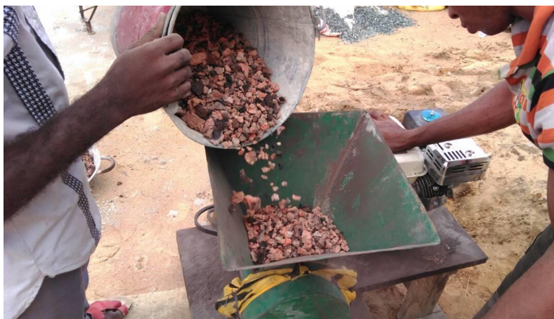
Plate 1: Grinding process of the chikoko Clay
