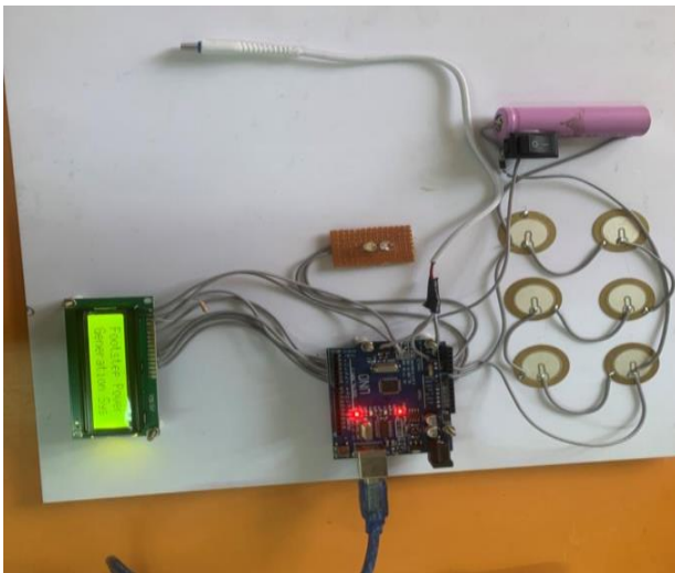
Figure 7.1 – Footstep power generation
