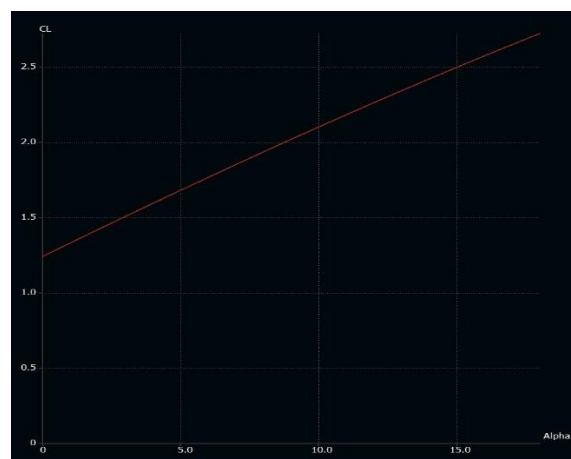
Fig. 10 Cl vs Cd, Cl vs Alpha and Cl / Cd vs Alpha for Upward Deflection of the Wing
