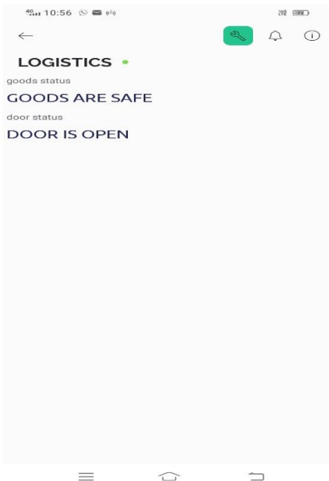
Fig 7: Blynk notification of current status
