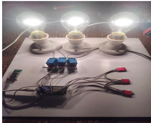
Figure 5.1 demonstrates the process of activating the light bulb using the smart touch switch panel.
