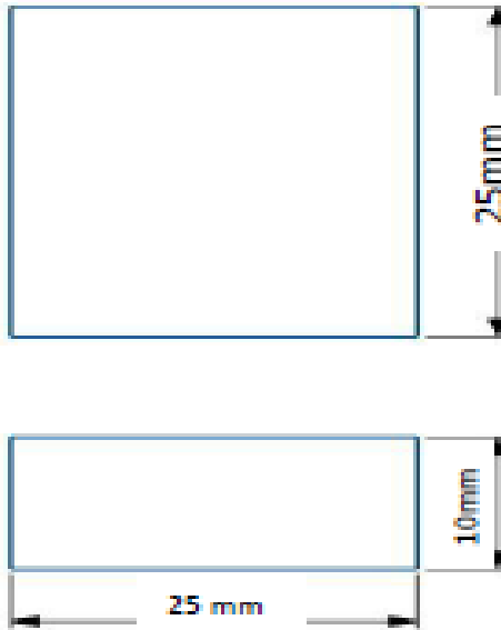
Figure 1 Geometry of Density Test Sample (All Dimensions are in mm)
