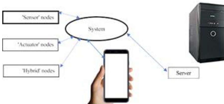
Fig. 2. The suggested structure of system of Internet of things.
