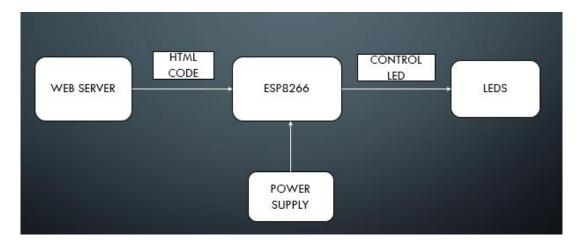
Figure 1: Here in data block the system block for ES8266 micro controller circuits has to be designed, that called as a web server. A web server which the HTML page, in order to provide a user interface for control LEDs. The action occurs as soon as the user interacts by means of web server, and sends HTML code containing LED control commands to be performed.
