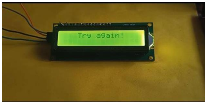
Fig 3: As the user placed the invalid finger or the unknown person is trying to unlock the door it is displaying try again on the LCD
