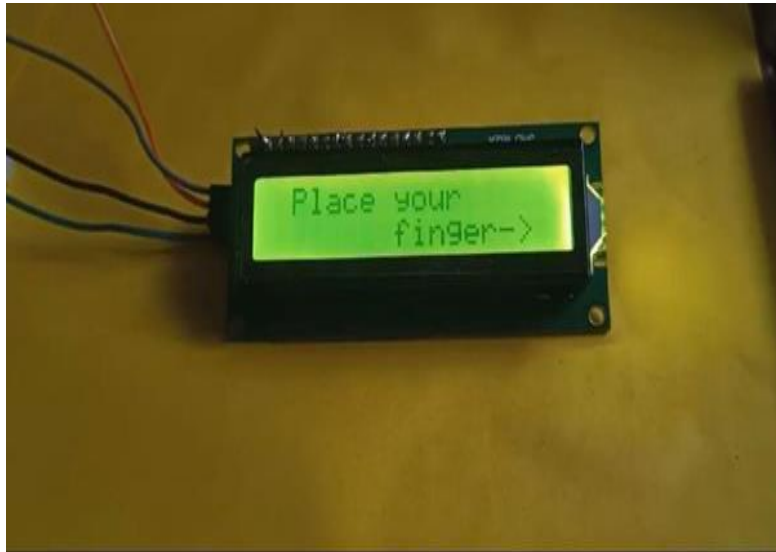
Fig 2: Asking the user to place the finger, Which is displaying on the LCD.
