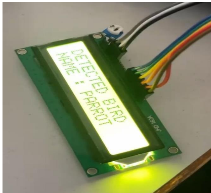
Fig 3. Bird is recognized and displayed on LCD
