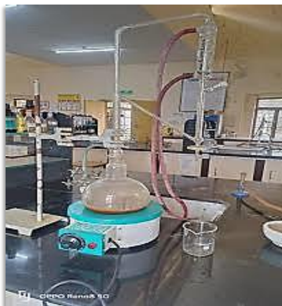
Fig.1.3: Extraction of clove oil from clove using Clevenger apparatus
