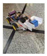
Case 2: Based on the color it starts following the line, if the is blue it turns left based on code and if the color is red it runs straight, if the color is green it turns right and follow through the end of the line.
