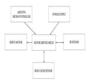
Figure 1 represents a color sorting and line-following robot. An Arduino microcontroller processes inputs from the RGB color sensor (for color detection) and the IR sensor (for line following). These signals control the motor driver shield, which operates the servo motor for sorting and navigation. A power supply powers the entire system.
