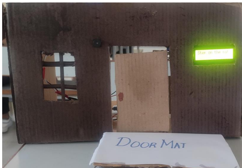
Case 1: When the authorized person stands on the door mat, the visitor is recognized via camera module and the door opens automatically.
