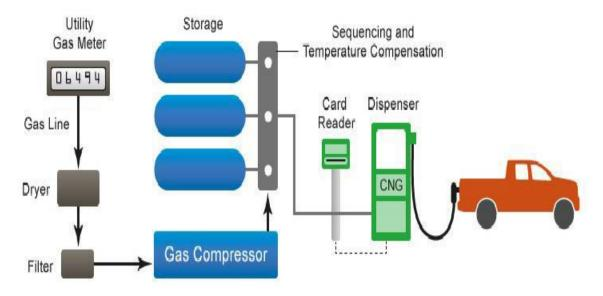
Fig 4 Fast filling station
