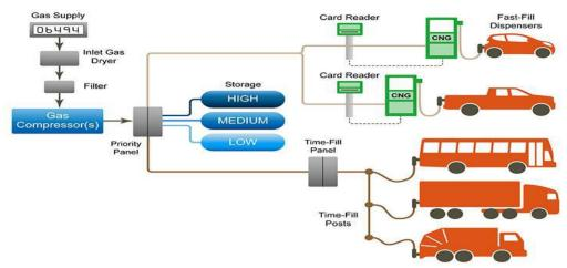
Fig 6 Combine Fast and time filling station
