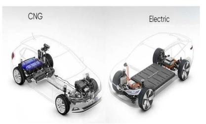
Fig 1. Arrangement of CNG and Electric Vehicles
