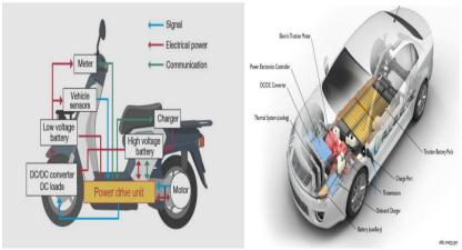
Fig 3. Electric Two wheeler and four wheeler vehicle
