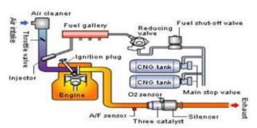
Fig 2. CNG fuel engine
