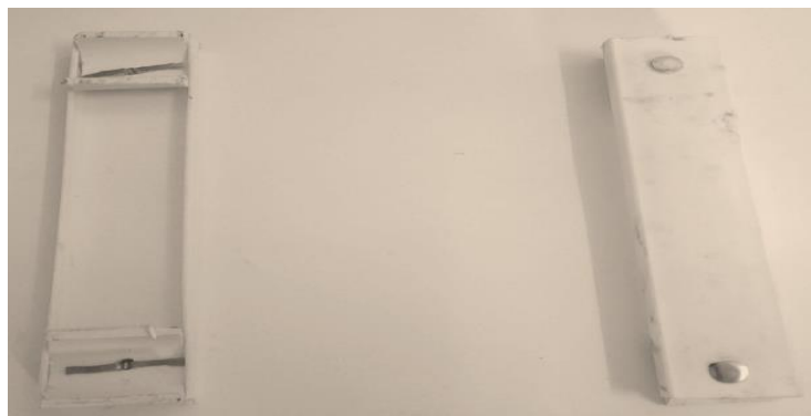
Figure 4.3: Specially Made Two Conductor Spacer
