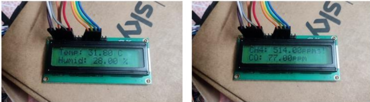
Fig.3 Display real-time gas concentration and temperature for user.
