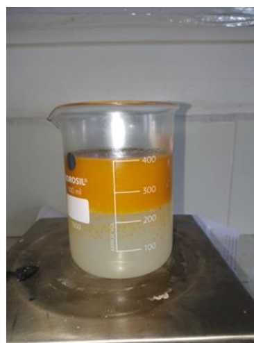
Fig f: Water-washed process for getting BD
