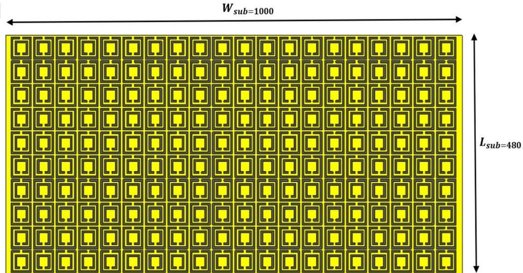
Fig.12. 200 Elements of CSSR Metasurface
