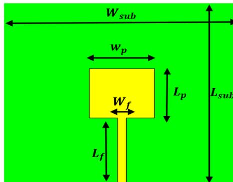
Fig 1: Simple patch antenna
