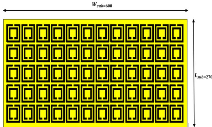
Fig.9. 60 Elements of CSSR Metasurface
