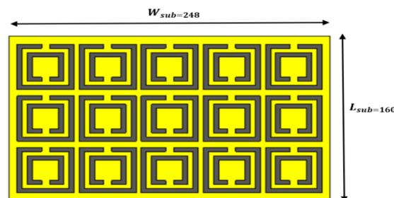
**Fig.7. 15 Elements of CSSR Metasurface**
