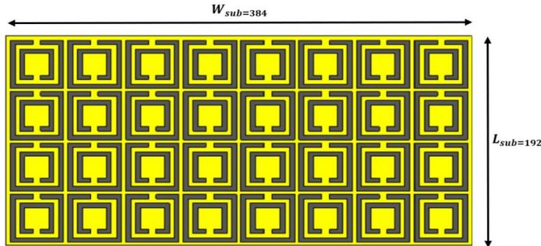
Fig.8. 32 Elements of CSSR Metasurface
