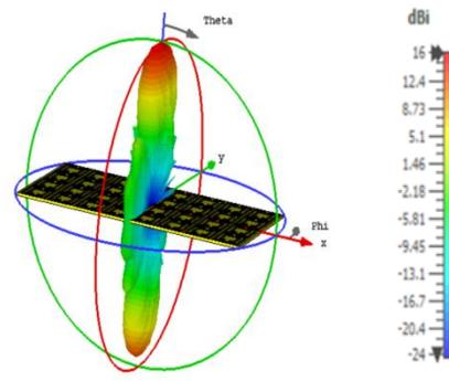
**(f): 3D Radiation Pattern****Fig. 3. Evolution stages of Graphene based metasurface**
