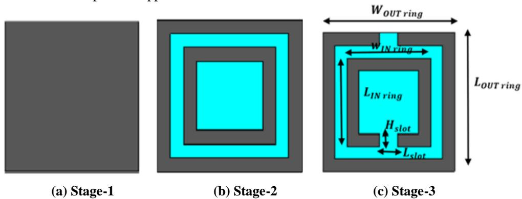
Fig. 2. Evolution stages of metasurface unit cell
