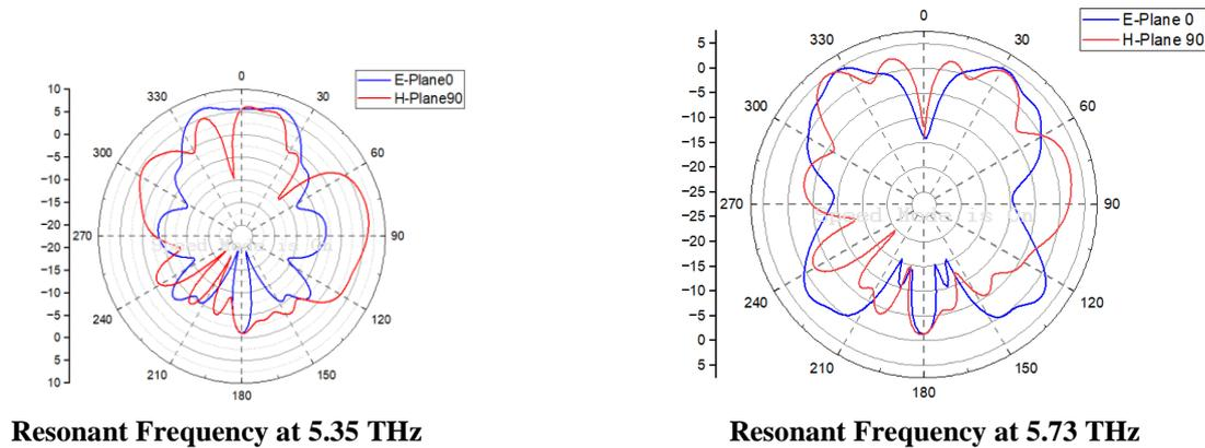
**Fig .6. Radiation Patterns for E-plane & H-plane**
