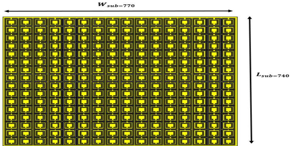
Fig.13. 256 Elements of CSSR Metasurface
