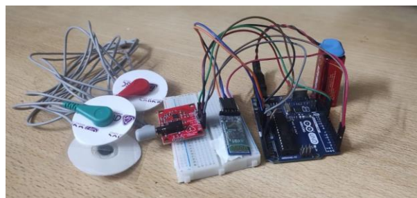
Fig 2 Hardware setup for real-time ECG collection
