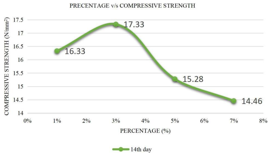
Graph 8.4 Graphical representation of compressive strength of blocks with surkhi and EPS beads at 14 th day
