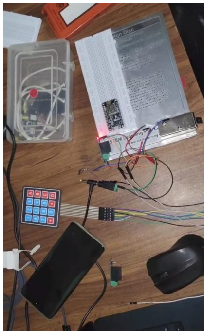
Fig 2: Keypad and solenoid lock connection
