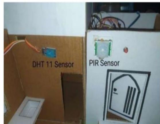
Fig. - Mounted DHT11 sensor and PIR sensor
