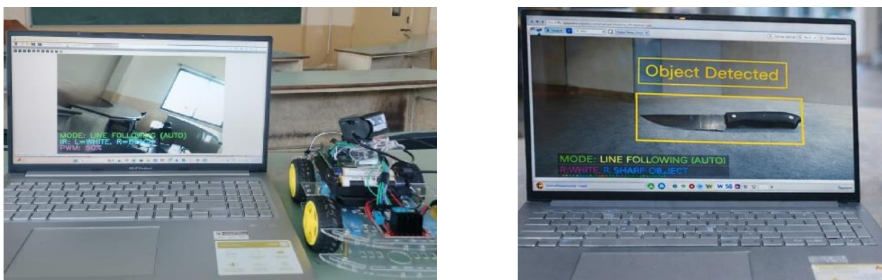
Fig. 4. Real-Time Object Detection Output Using MobileNet SSD on COCO Dataset and Live Video Streaming from Raspberry Pi Camera via VNC Viewer
