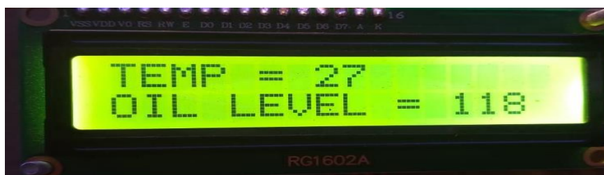
(LCD display showing transformer temperature and oil level under normal operating conditions)
