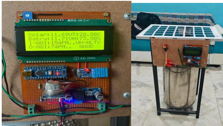
Fig.:10 PROTOTYPE OUTPUT LCD Display showing Air Quality Readings
