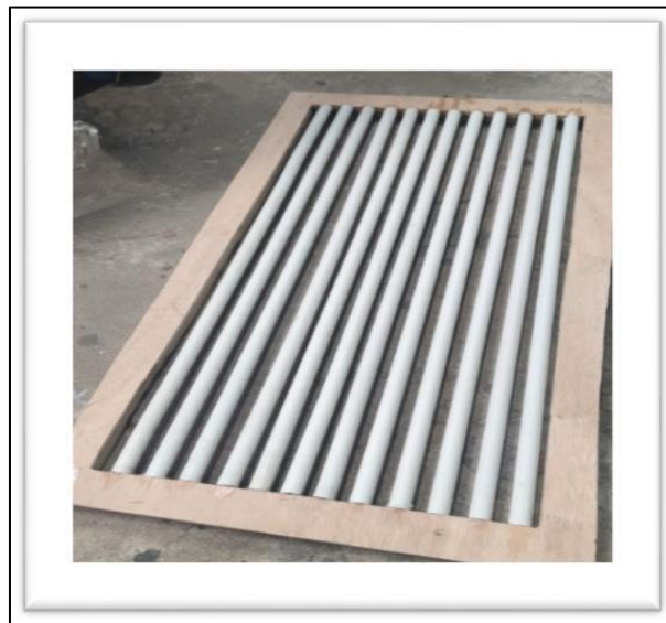
Fig.3: Plenum Chamber Construction
