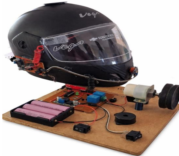
Figure.1: The IoT-based smart and safety helmet
