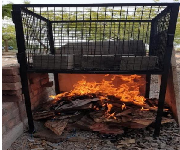
Figure 01: Fire testing of Concrete Cube Specimen
