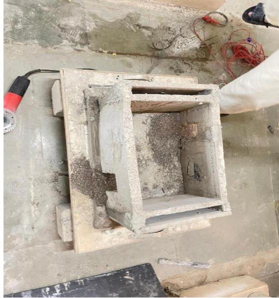
Figure 1: Cavity Wall Model
