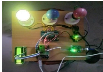
Fig.10. Normal condition In the above figure, the green bulb is glowing that indicates the water quality is normal. The sensors have detected that water quality parameters like pH, temperature, TDS, NH 3 and turbidity are within the optimal range. Then the system gives the visual result in LCD display as normal.
