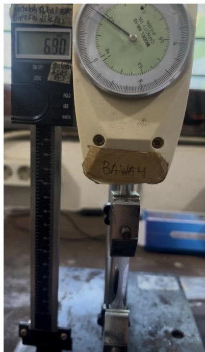
Figure 2: Manual tensile testing apparatus used in this study. The specimen is gripped between the lower fixed clamp and the upper crosshead linked to the analog force gauge (model NK-10, 10 N). Crosshead displacement is recorded by the digital dial indicator on the left.
