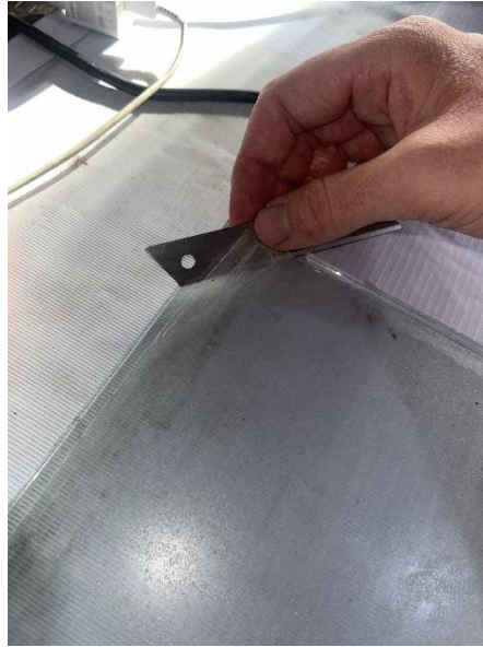
Figure 1: Dried white Eucheuma cottonii bioplastic film on the glass casting plate, prior to being cut into specimens. The film is approximately 0.2 mm thick. Dogbone specimens with the geometry described in Section 2.3 were hand-cut from the central region of the film with a scalpel and a metallic template.
