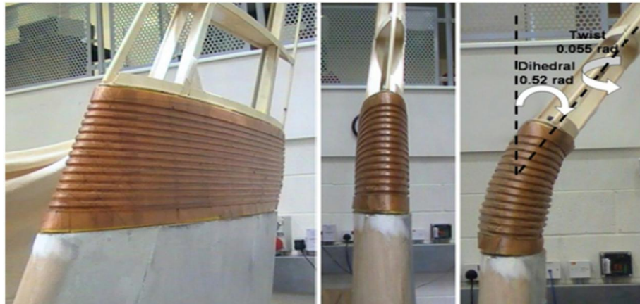
Figure 14. Demonstration of extension and canting of a morphing winglet with a corrugated structure [57]
