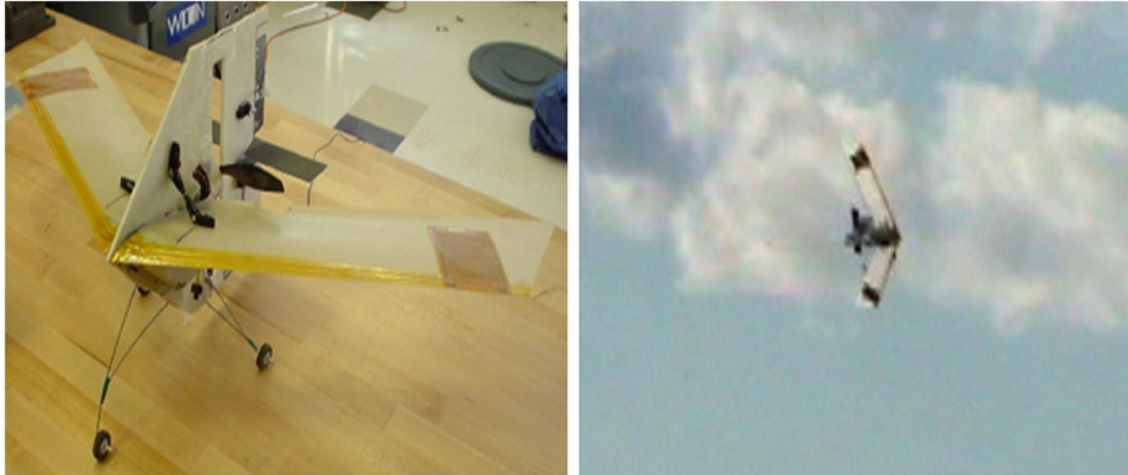
Figure 5. Micro air vehicle controlled by piezoelectric materials on the ground and in flight [23]
