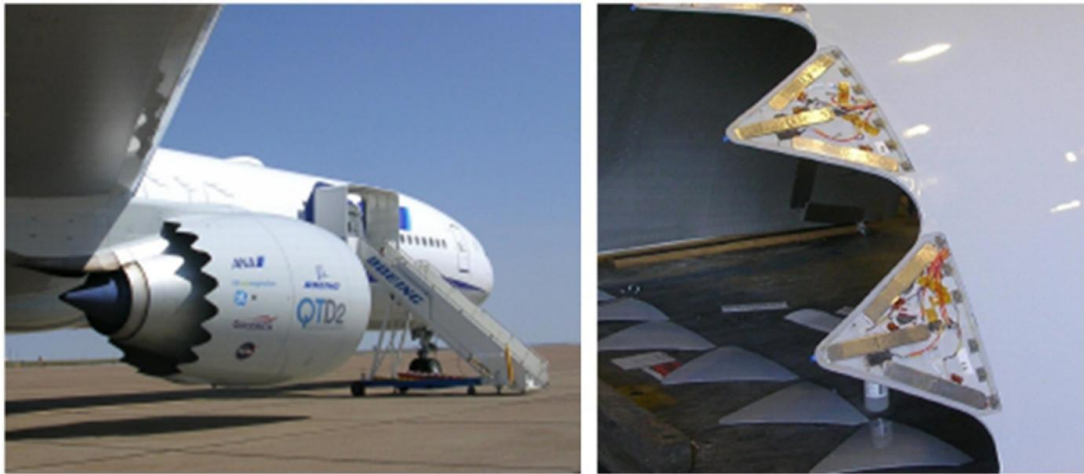
Figure 5. Full-scale flight tests of SMA-actuated variable-geometry chevrons on a Boeing 777-300ER
