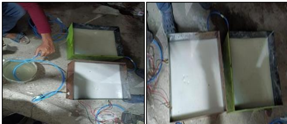
Figure 3.2: Box type Heat Exchanger and Paraffin Wax Chamber
