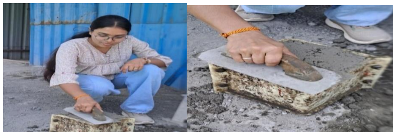
Fig No 2: Cube Casting Process
