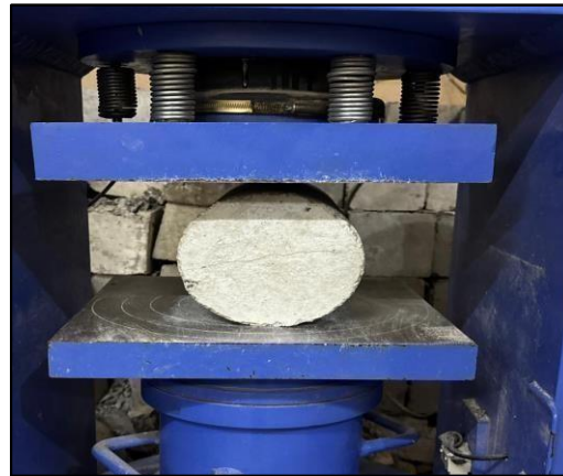
Fig. No. 2 Split Tensile Strength Test On Compressive Testing Machine
