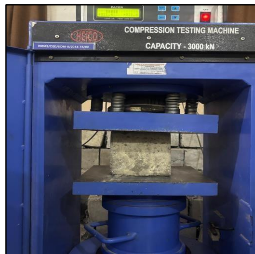
Fig. No. 1 Compressive Test On Compressive Testing Machine Split Tensile Strength Test
