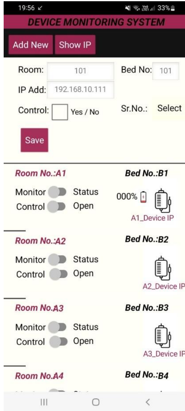
Figure 3: Android Application Interface for Saline Bottle Device Monitoring and Control.
